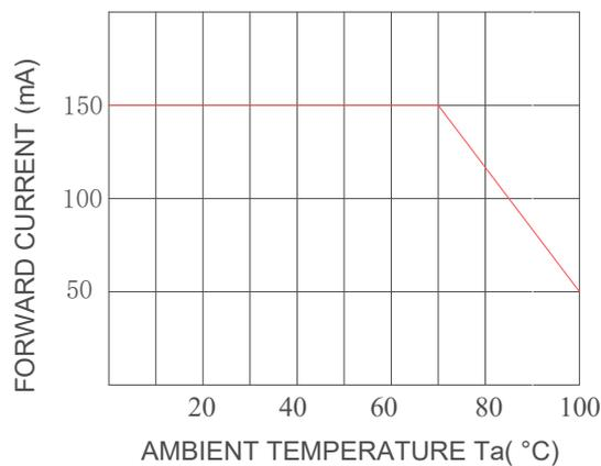
◆ 温度与亮度关系 (Temperature and brightness characteristic)
